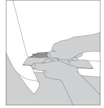
Carefully cut the excess with your utility knife. Place your plastic squeegee between your knife and the window frame to help cut straight.
