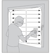
Use the squeegee to adhere the Squid<sup>®</sup> against the glass. Press the Squid<sup>®</sup> in the middle and rub all air and creases away from the center outwards (see arrows). Press the entire surface, all edges and corners well with the squeegee.
